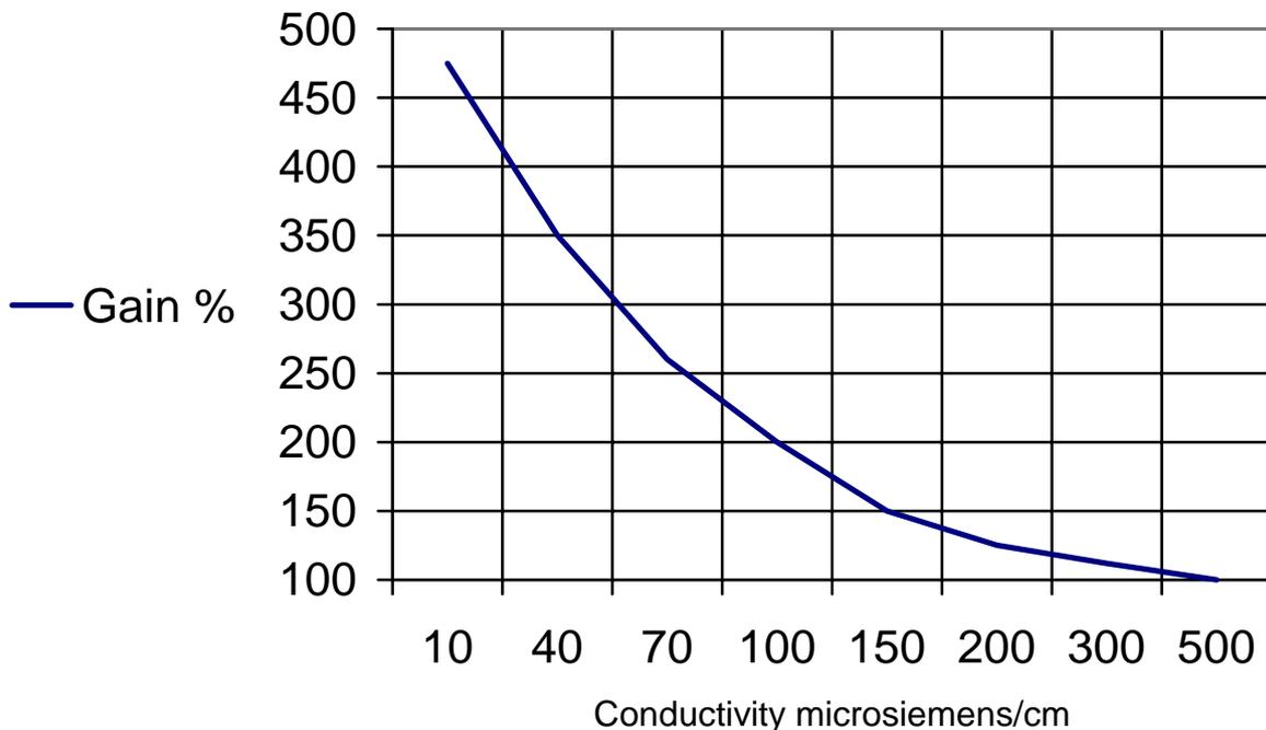
On delivery, the fish counter has this compensation curve established as a default set of parameters and will refer to it in the set-up procedure prior to normal operation.
